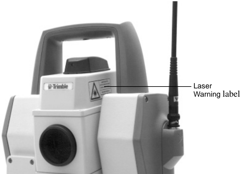
Figure 1.10 Laser warning label location
