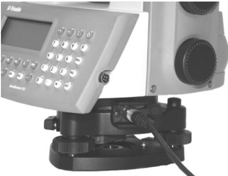
Figure 1.4 Connecting the external battery to the instrument.
