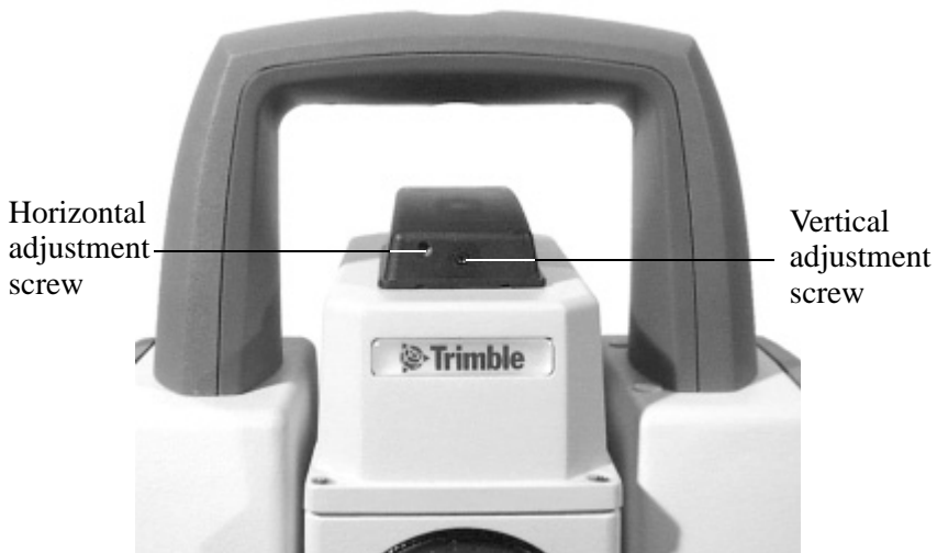
Figure 8.2 Laser Pointer adjustment screws
