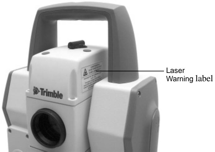
Figure 1.7 Laser warning label location
